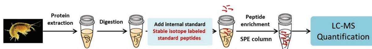
Figure II-10 – Main stages of sample preparation for SRM analysis. SPE – solid phase extraction.
